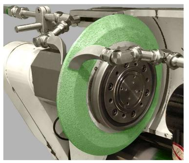
The flow-optimized needle nozzles and the 3D-printed nozzles are each available in left and right versions. To ensure efficient and collision-free lubricoolant supply to the grinding zones, the nozzles are designed for different module ranges.
