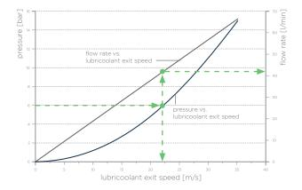
Starting with the pressure, you directly find the associated lubricoolant exit speed. The grey line enables you to then determine the correlation between the lubricoolant exit speed and the associated lubricoolant flow rate.
