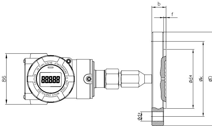
**Example of PAS remote assembled with diaphragm seal and capillary**
